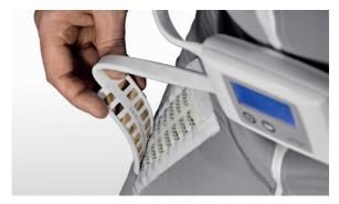
6. Thread the belt through the loops on the back of the control unit and secure the control unit and belt around the waist. Then secure the magnetic couplings on the garment in accordance with the picture above. Ensure that they are positioned correctly.
